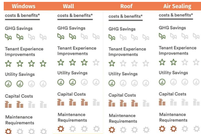
Figure 4: Envelope Improvement Costs & Benefits from New York City Accelerator and Building Energy Exchange. Cost and benefits of window, wall, and roof insulation and air sealing at room ACs, assuming all existing aspects of the envelope are minimally compliant. Ratings are determined by industry experts and calculated relative to the system end use, not the whole building.
