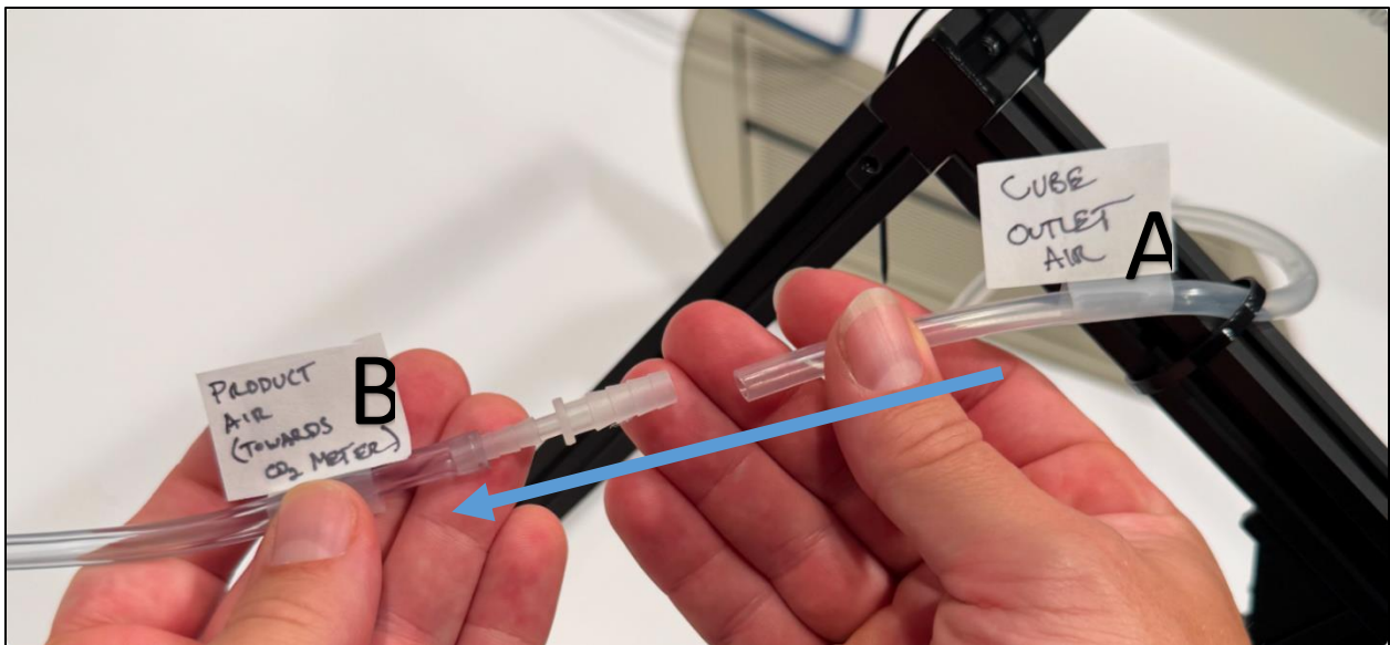
Figure 4: Connection Points for Cube Outlet. Point A is the Cube Air Outlet. Point B is the connection source to the CO 2 meter and rotameter that will be provided during the competition. Air will flow in the direction shown by the blue arrow.
