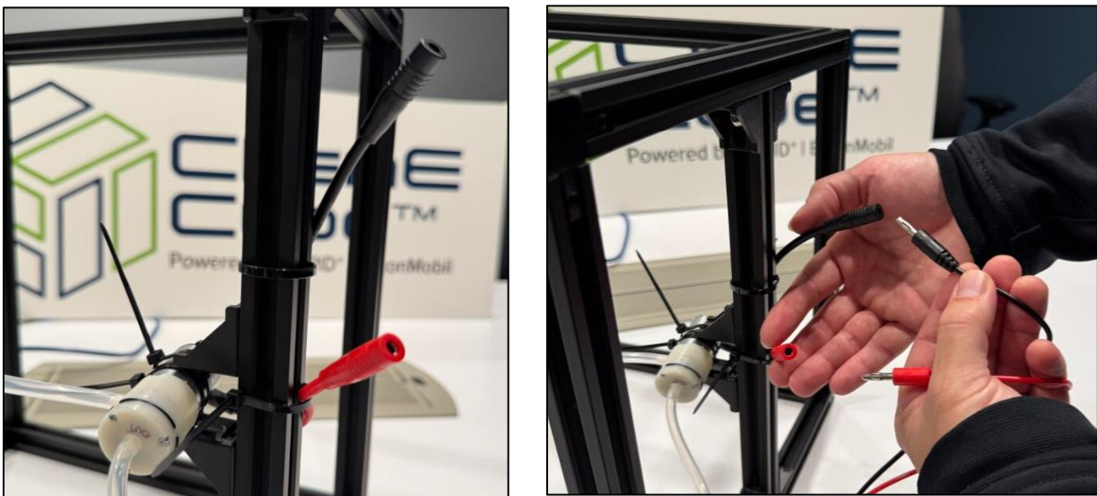
Figure 2: Connection Points for Power for Cube - Notice the example cube is providing female banana jack connections.
