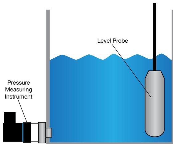
▲ **Figure 6.** The water level in a tank can be measured indirectly by a pressure sensor. Because the pressure of water increases 100 mbar for every meter of water depth, the water level can be derived based on pressure differences. Alternatively, a level probe can be used.
