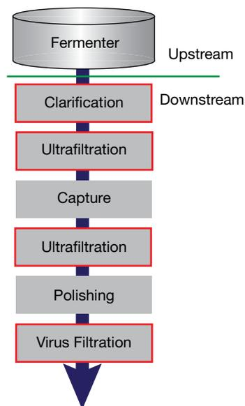
► **Figure 10.** A typical bioprocess consists of an upstream fermenter followed by multiple downstream separation steps. Membrane processes may be used for the operations outlined in red — clarification (often a combination of centrifugation and microfiltration), ultrafiltration, and virus filtration.
