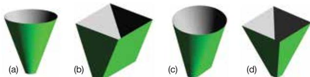
▲ **Figure 1.** Common geometries for hoppers, bins, and silos include (a) conical, (b) wedge, (c) transition, and (d) pyramidal.
