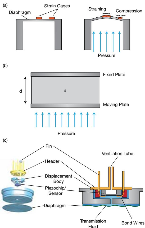
▲ **Figure 1.** Pressure sensors measure the deflection of a diaphragm or membrane that is acted on by a force and convert the amount of deflection into an electronic signal. In resistive pressure sensors (a), strain gages pick up changes in pressure by bending or compressing. In capacitive pressure measurement (b), the distance between two membranes changes with a change in fluid pressure. In piezo-resistive sensors (c), oil transmits pressure to the sensor chip via an external diaphragm.
