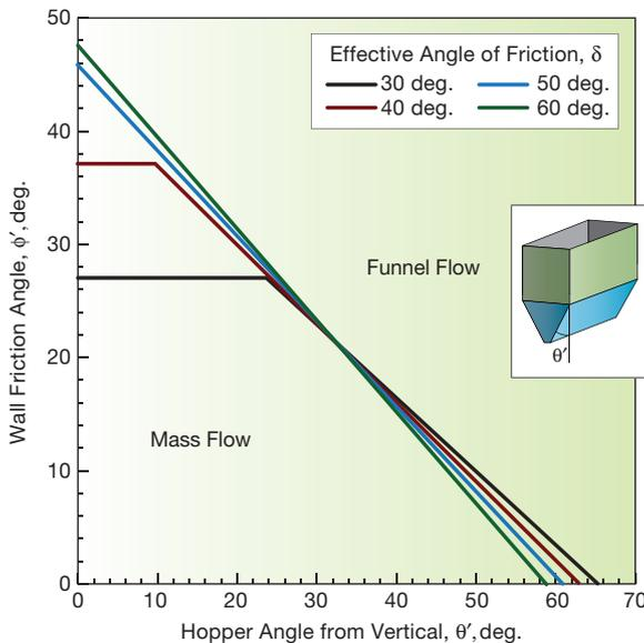
▲ **Figure 9.** Wedge-shaped outlets for mass flow have hopper angles ( $\theta'$ ) that are typically 10 deg. less steep than those of conical hoppers.
