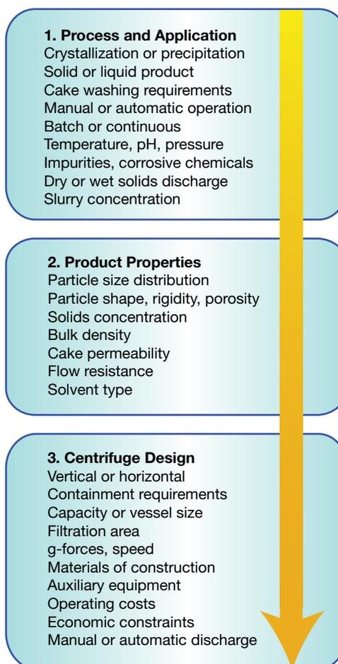
▲ **Figure 1.** The three-step process for centrifuge selection begins with an evaluation of the process and product properties, and then an assessment of centrifuge options.
