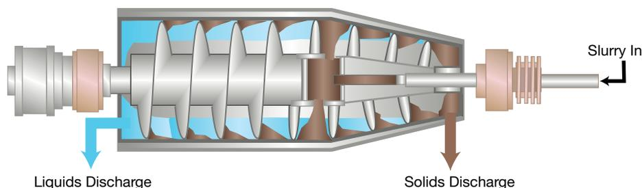
▲ **Figure 9.** A cross-sectional view of a decanter shows the movement of liquids and solids via high rotational forces.
