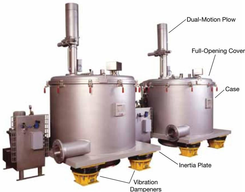
▲ **Figure 3.** The vertical basket bottom-discharge centrifuge may be suitable for hazardous substances, as it offers better containment.
