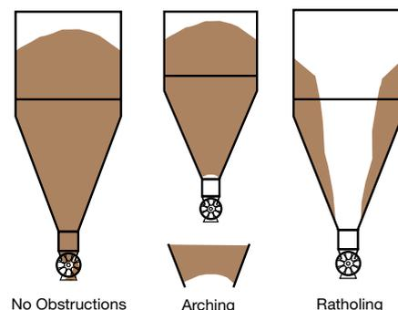
▲ **Figure 7.** Obstructions such as cohesive arches and ratholes prevent flow through a hopper.
