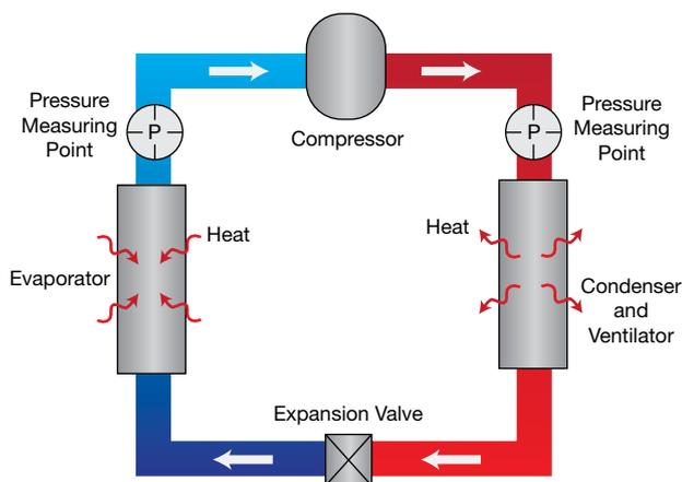
▲ **Figure 7.** In a typical refrigeration cycle, liquid absorbs heat when it changes from liquid to gas, and gas gives off heat when it condenses from gas to liquid. Pressure is typically measured both before and after the refrigerant passes through the compressor.
