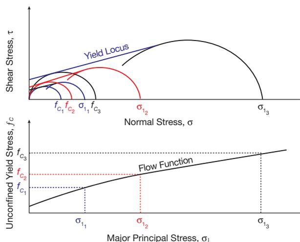
▲ Figure 3. The flow function is the relationship between the major stress and the unconfined yield strength. A graphical representation is constructed by connecting the points of different yield locus measurements.
