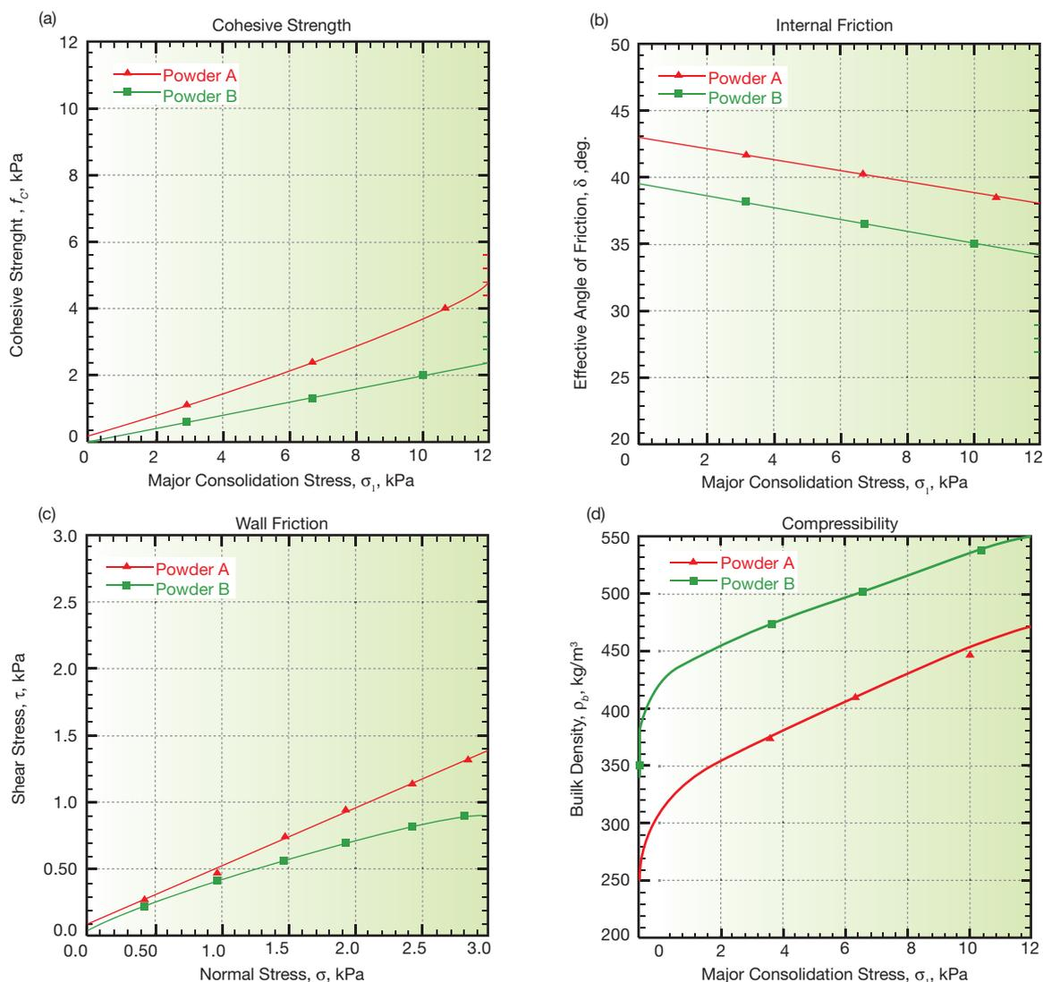
▲ **Figure 14.** Fundamental flow properties of Powders A and B for the sample design calculations.
