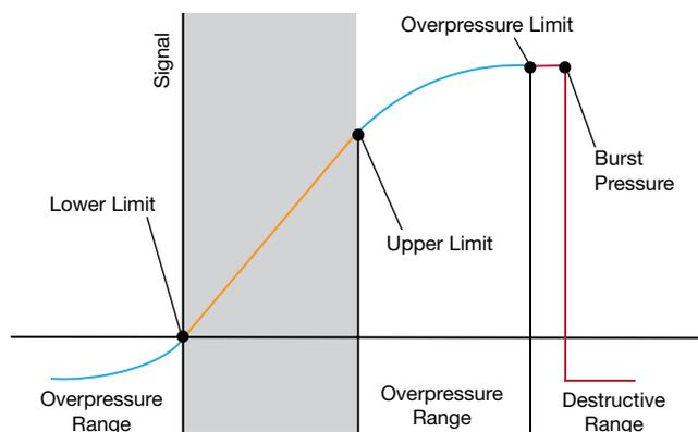
▲ **Figure 4.** A sensor's pressure range (gray region) defines the lower and upper limits of pressure measurement, as well as the overpressure range.
