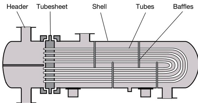
▲ **Figure 1.** In shell-and-tube heat exchangers, heat is transferred across the tube walls separating the hot and cold streams.
