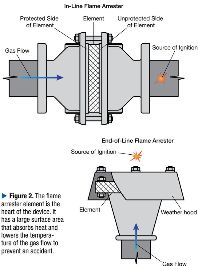
◀ **Figure 1.** When specifying a flame arrester, use the appropriate terminology to ensure you purchase the correct arrester type.
