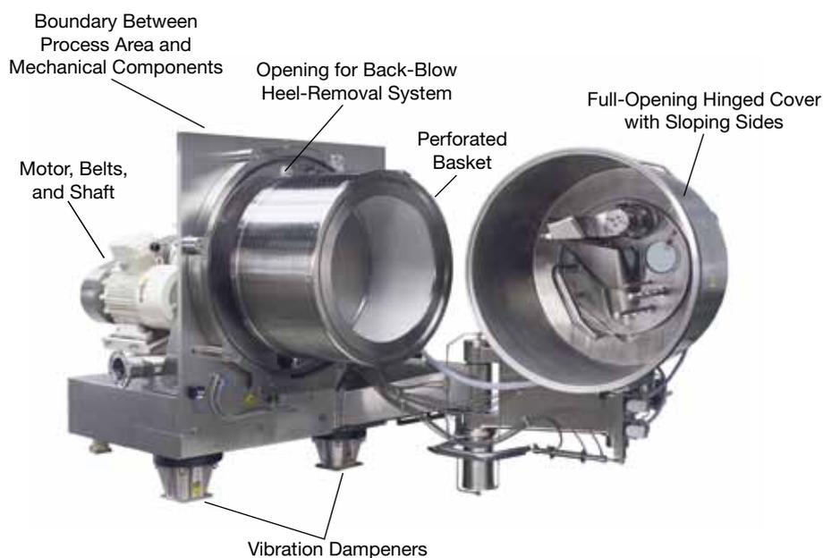
▲ **Figure 6.** A horizontal peeler for pharmaceutical applications features a CIP system and discharge chute for sanitary operation.
