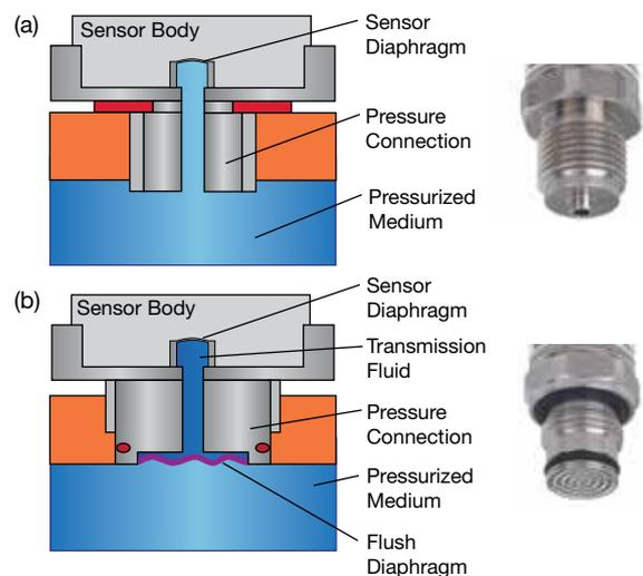
▲ **Figure 3.** In an internal-diaphragm connection (a), the process fluid comes in direct contact with the sensor diaphragm through a pressure port. In a flush-diaphragm connection (b), an additional stainless steel diaphragm is in contact with the process fluid, and a transmission fluid transmits the pressure to the internal diaphragm.
