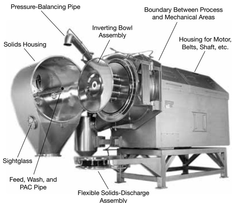
◀ **Figure 7.** An inverting filter centrifuge is the most versatile of all centrifuges and allows for cake thicknesses less than 1/2 in.
