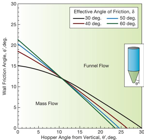
▲ **Figure 8.** When designing a hopper with round or square outlets, select a hopper angle ( $\theta'$ ) that falls to the left of the appropriate curve.
