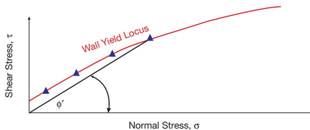
▲ Figure 5. The wall yield locus is constructed by plotting shear stress against normal stress.
