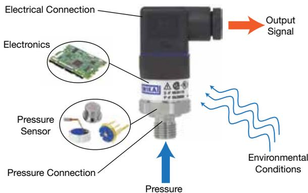
▲ **Figure 2.** A typical pressure transmitter is a fully standardized instrument that contains a pressure connection, a sensor, electronics, and an electrical connection, and outputs a standard electrical signal.
