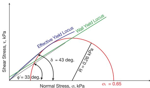
▲ **Figure 15.** A Mohr's circle is used to determine the wall friction angle from the effective yield locus and wall yield locus.
