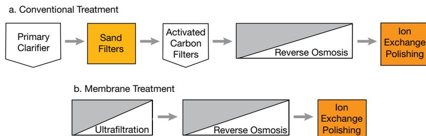
▲ **Figure 9.** Conventional boiler feedwater treatment (a) involves more steps than the hollow-fiber UF and RO water treatment process (b).
