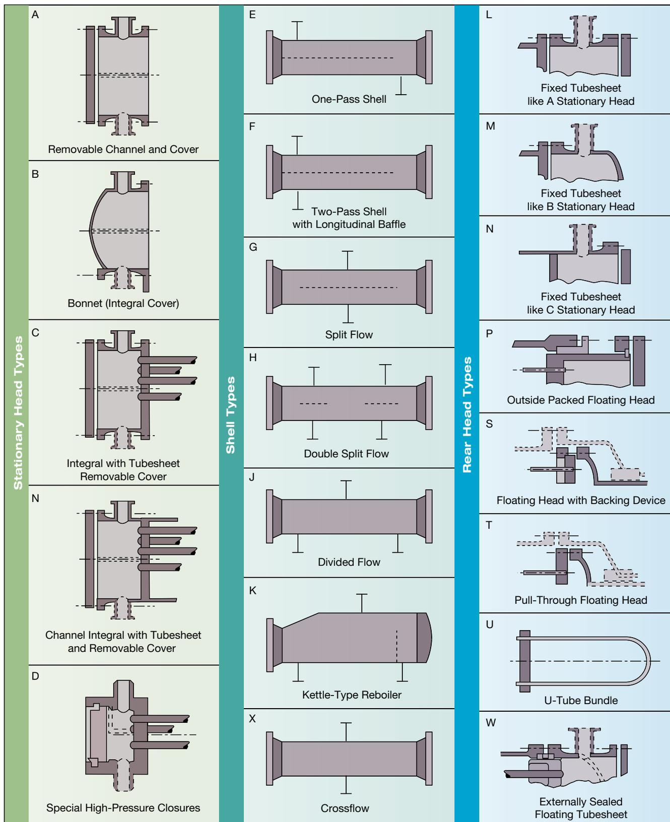
▲ **Figure 2.** TEMA's notation system designates a shell-and-tube heat exchanger's type of front head, shell, and rear head.
