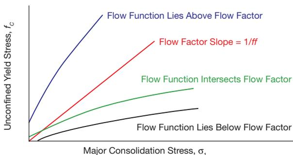
▲ **Figure 12.** To determine if a critical stress exists and a cohesive arch is likely to form, the flow function and flow factor are plotted on the same graph.
