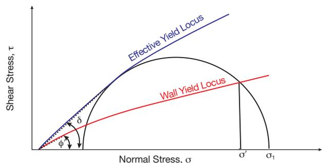
▲ **Figure 10.** The angle of wall friction and effective angle of friction are found by plotting the effective yield locus and wall yield locus.
