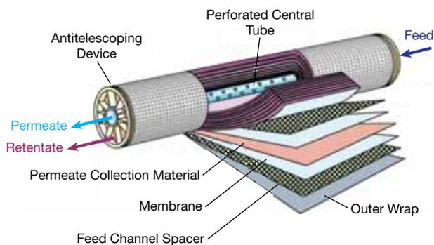
▲ **Figure 7.** Spiral-wound membrane modules are constructed by rolling a multilayer assembly of flat-sheet membranes and spacer screens around a perforated tube and sealing the membrane/spacer layers on three sides.
