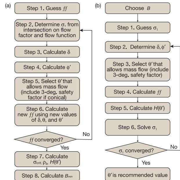
▲ **Figure 13.** (a) When the flow function and flow factor intersect, follow the steps in the flowchart on the left to determine the critical hopper outlet size and recommended mass flow hopper angle. (b) Use the flowchart on the right to find the recommended hopper angle for mass flow for a hopper with a known outlet dimension ( $B$ ).
