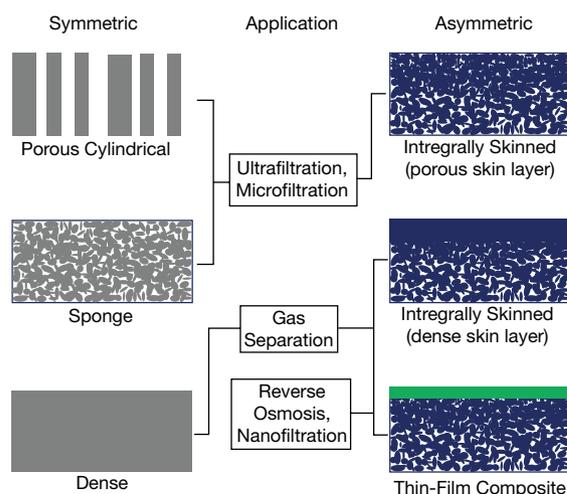
▲ **Figure 4.** Membrane structures may be symmetric or asymmetric. Membrane morphologies include porous cylindrical, sponge, and dense (symmetric); and integrally skinned and thin-film composite (asymmetric) (10).
