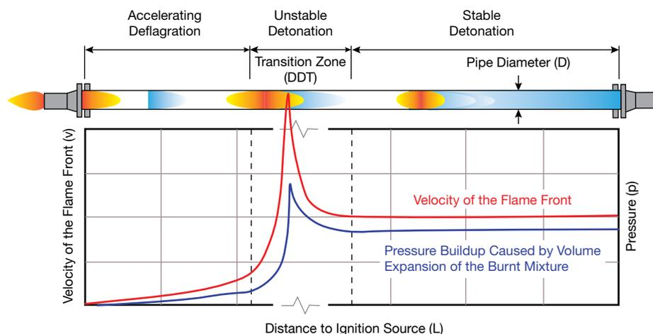
▲ **Figure 7.** As explosions propagate within a piping system, they transition from an accelerating deflagration to an unstable detonation and, finally, to a stable detonation.
