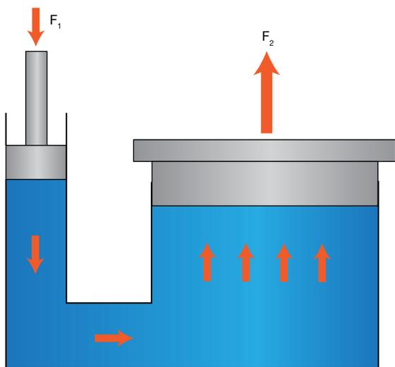
▲ **Figure 5.** In indirect force measurement, a system's known geometry can be used to calculate force based on pressure measurements. In this figure, two movable pistons are in contact with hydraulic oil. If the smaller piston moves down, the larger piston is pushed up with a greater force. Measuring the pressure exerted by the small piston allows the force to be calculated.
