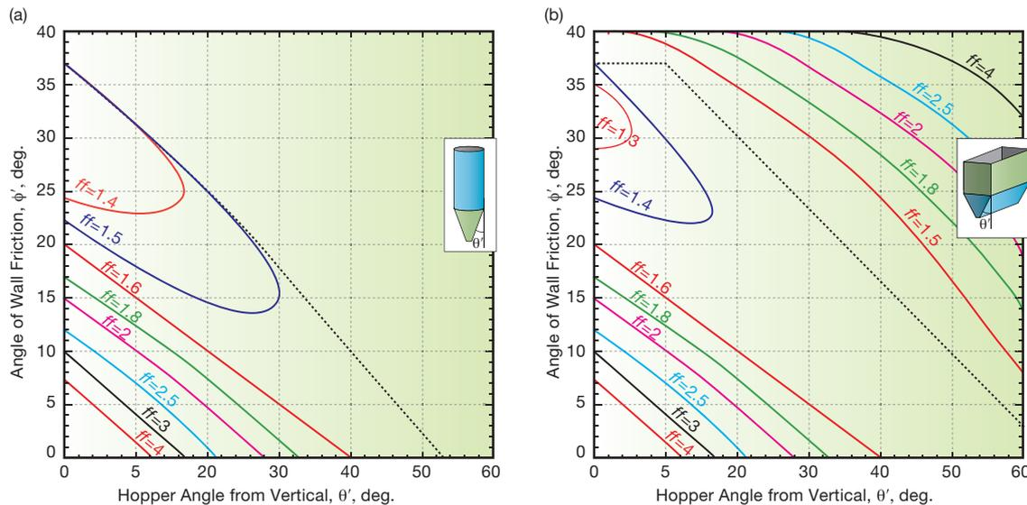
▲ **Figure 11.** The flow factor ( $ff$ ) depends on the hopper angle from the vertical ( $\theta'$ ), the wall friction angle ( $\phi'$ ), and the effective angle of friction ( $\delta$ ). These sample charts are for (a) conical hoppers and (b) planar flow hoppers with rectangular outlets; for both, the effective angle of friction  $\delta = 40$  deg. The dotted line represents the boundary between mass flow and funnel flow. Source: Adapted from (3).
