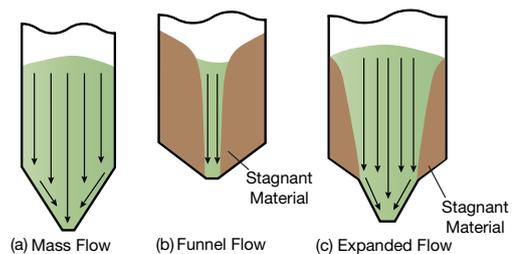
▲ **Figure 6.** Mass flow (a) ensures a more-uniform discharge of bulk solids than funnel flow (b) or expanded flow (c).
