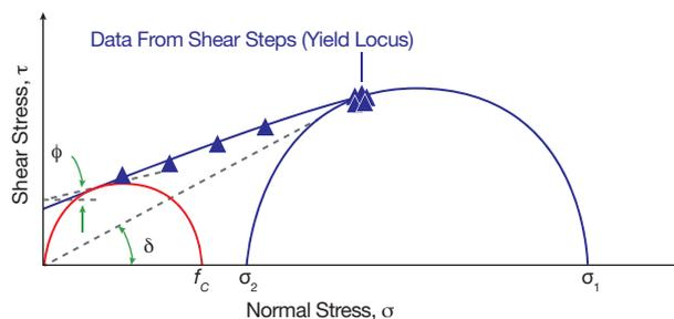
▲ **Figure 2.** The yield locus, determined by the shear cell tests, is used to calculate the major principal stress ( $\sigma_1$ ), unconfined yield strength ( $f_c$ ), effective angle of friction ( $\delta$ ), and kinematic angle of internal friction ( $\phi$ ).
