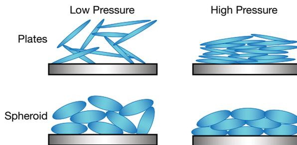
▲ **Figure 2.** Compact cakes have smaller voids between particles, which limits filterability.
