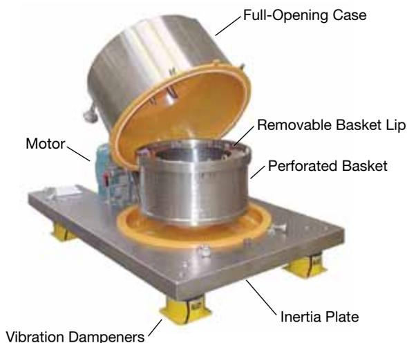
▲ **Figure 4.** This cGMP vertical basket centrifuge has a full-opening cover to allow complete sanitization of all internal surfaces.
