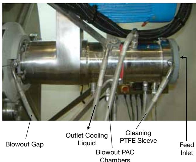
▲ **Figure 8.** Pressure-added centrifugation (PAC) uses pressure as its driving force to help dry the solid cake.
